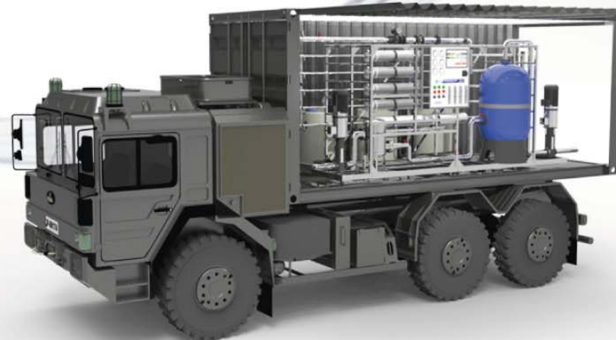
Mobile water treatment system
